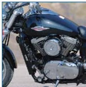
*This engine differs from the Classic's left with 37mm instead of 33mm intake valves, bigger intake ports, 40mm instead of 36mm injector throats and new cam profiles.*
