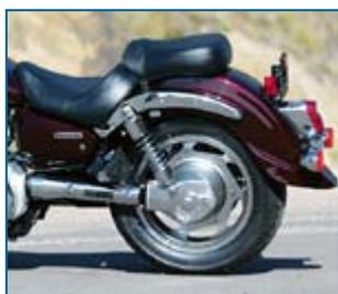
*Like the Suzuki, the Kawasaki uses shaft final drive, which is heavier and creates more drivetrain lash than a belt. Some see it as more reliable, though.*
