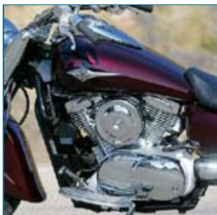
*Introduced last year, the Kawasaki 1600 engine is an 82cc expansion of the 1500 with extensive changes throughout. Details like the unsightly horn grate on us.*
